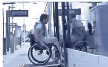
All stations feature barrier-free entry as special kerb stones allow close platform docking.
